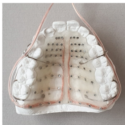
Figure 3. (a) A thermoformed EPG plate (displayed on a dental plaster cast) that shows the comparison of two types of electrode placement, i.e., the use of pre-tested flexible circuits (left) and the conventional method of individual electrode placement (right); (b) a pre-tested flexible circuit (right) comprised of electrodes (left) embedded on an electrode sheet (middle); and (c) a Mcyam EPG plate.
